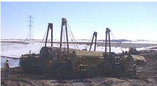
A tank car being off loaded to be buried in the industrial landfill.
