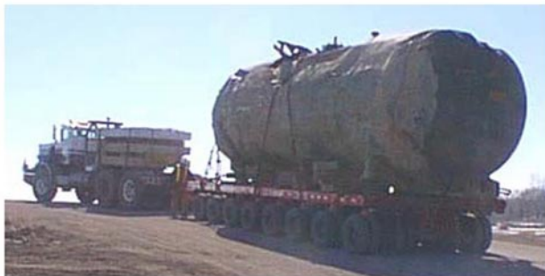
Perkins transporter moving a damaged tank car to its final destination in a landfill in IGH, MN
